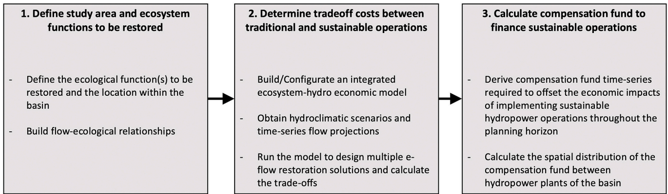
Fig. 4. Steps applied to simulate the electricity market as a cost-sharing mechanism to implement sustainable hydropower operations.
